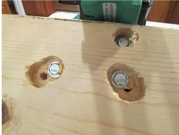
Countersunk holes on bottom of base
